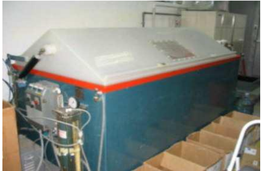
Salt Spray Chamber per ASTM B117
